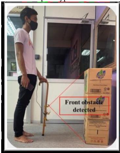
b) Experiment on prototype when an object is in front of a visually impaired person
