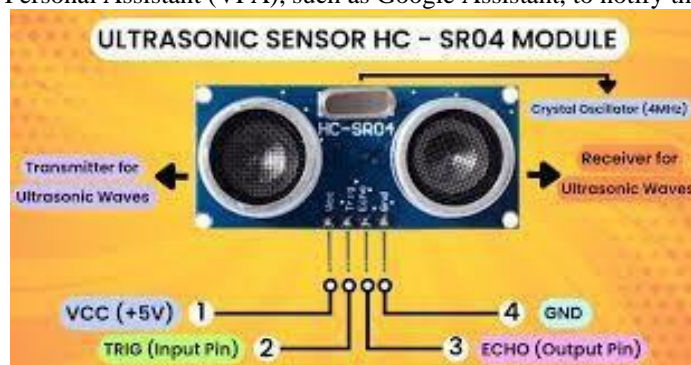
Figure 5: Pins on HC-SR04 ultrasonic sensor
